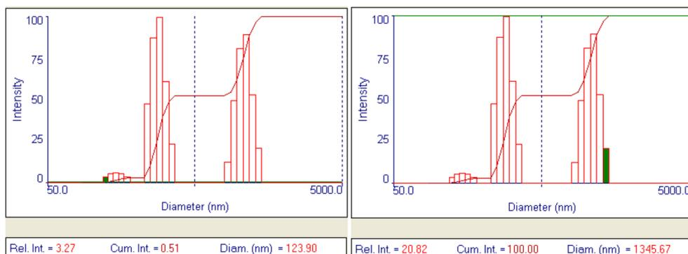
Fig. 1. Histogram of schungite particles distribution according to their sizes after the USD in water during 15 minutes
