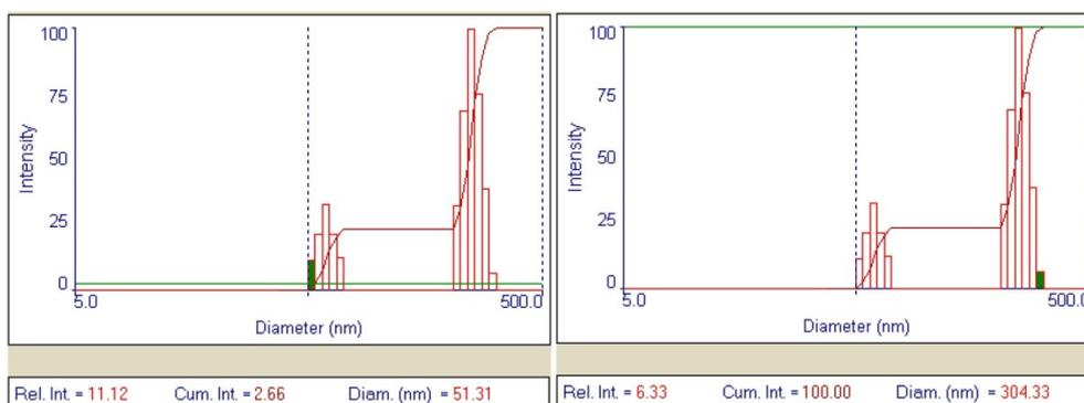
Fig. 3. Histogram of schungite particles distribution according to their sizes after the USD in water during 15 minutes in the presence of NF stabilizer
