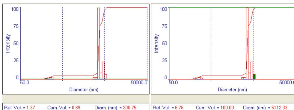
Fig. 2. Histogram of schungite particles distribution according to their sizes after the USD in water during 30 minutes
