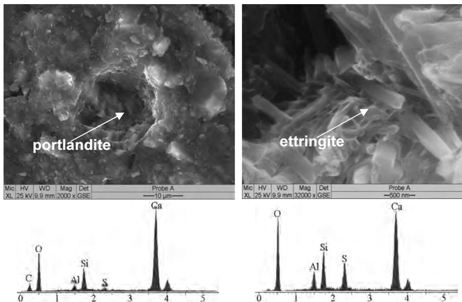
Fig. 5. The SEM images and the EDX spectrum of multicomponent cement
