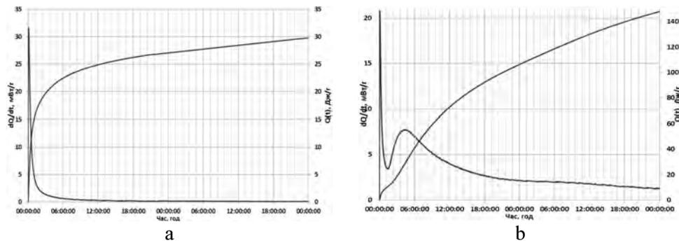
Fig. 3. The heat of hydration of Roman cement (a) and multicomponent cement (b)
