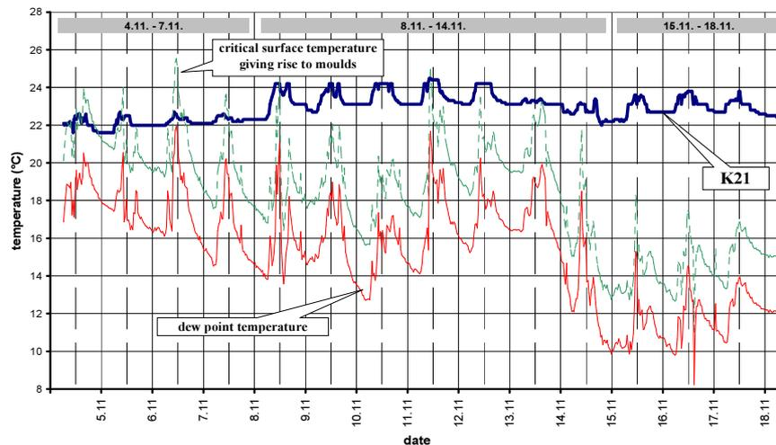
Fig. 6. Changes of indoor surface temperature in the upper part of kitchen office inner wall compared to the critical temperature of mildew occurrence and the dew point temperature
