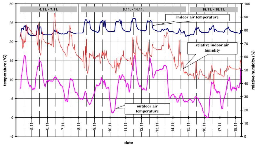
Fig. 5. Changes of indoor atmosphere temperature and relative humidity in the kitchen office and of the outside atmosphere temperature during the measurements
