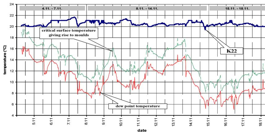
Fig. 4. The changes of indoor surface temperature in the upper part of the peripheral wall in the manager's office compared to the critical temperature of mildew occurrence and to the dew point temperature
