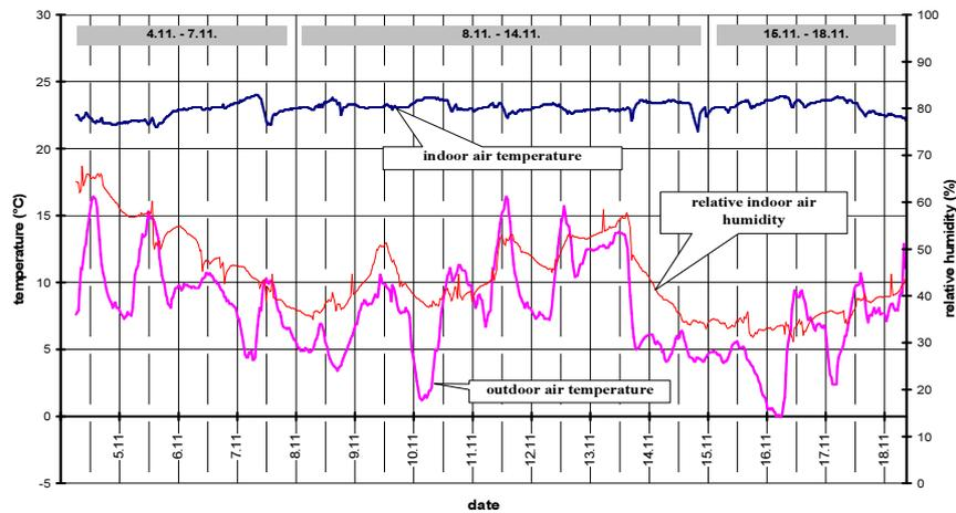
Fig. 3. Temperature and relative humidity of the indoor air in the room of manager's office and outside air temperature changes during measurement
