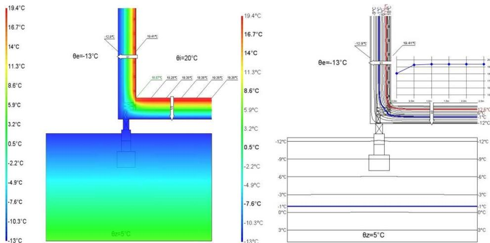
Fig. 10. Results of 2D modeling of detail and course of temperature
