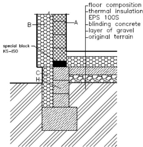
Fig. 3. Establishment with special block, with plinth insulation
