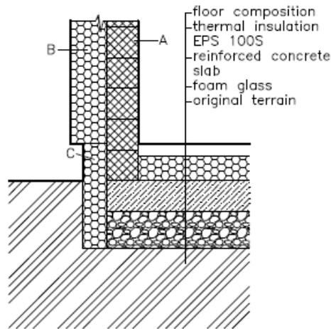
Fig. 5. Establishment on brush of foam glass
