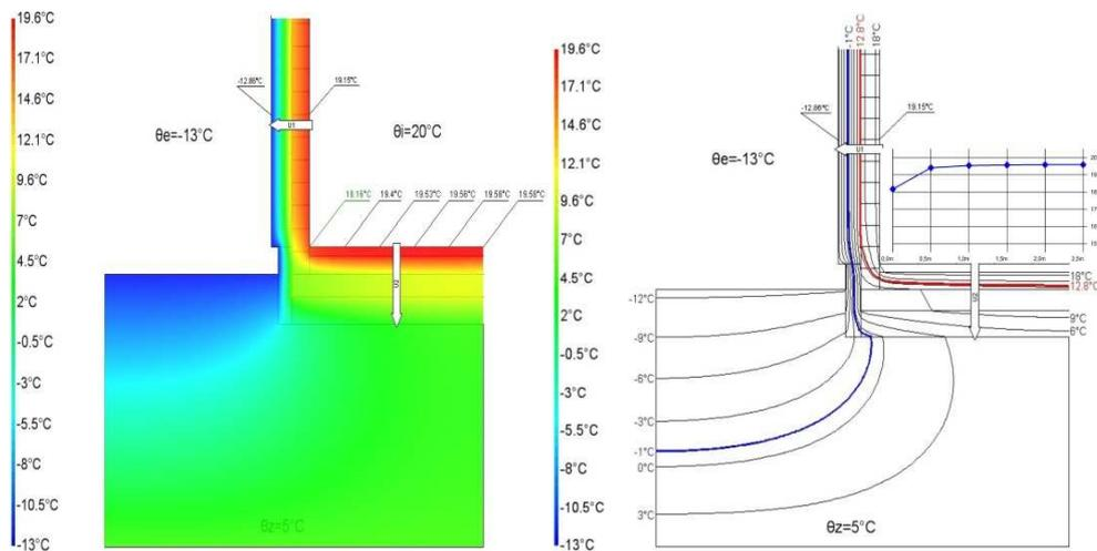
Fig. 6. Results of 2D modeling of detail and course of temperature
