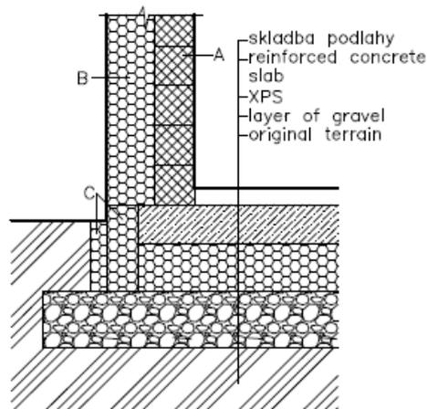
Fig. 7. Establishment on tub of extruded polystyrene boards
