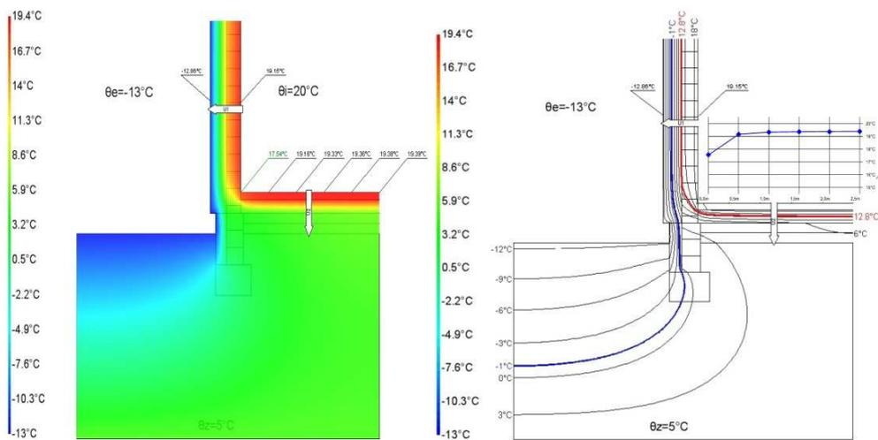
Fig. 4. Results of 2D modeling of detail and course of temperature
