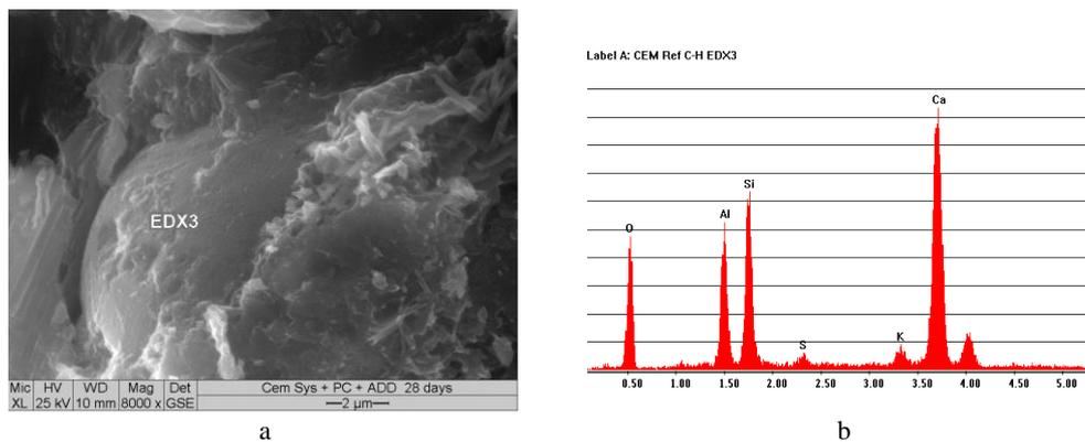
Fig. 8. Microstructure (a) and EDAX spectrum in spot EDX3 (b) of cementitious system with finely ground fly ash after 28 days of hardening
