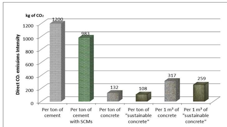
Fig. 1. Typical direct CO<sub>2</sub> intensity - cement and concrete
