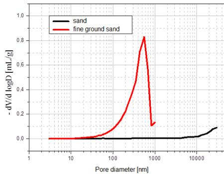
Fig. 3. Cumulative pore volume of sand and finely ground sand
