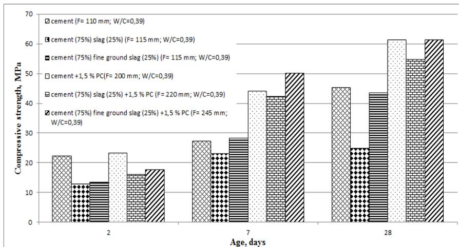
Fig. 6. Compressive strength of fine grained concrete with BGFS
