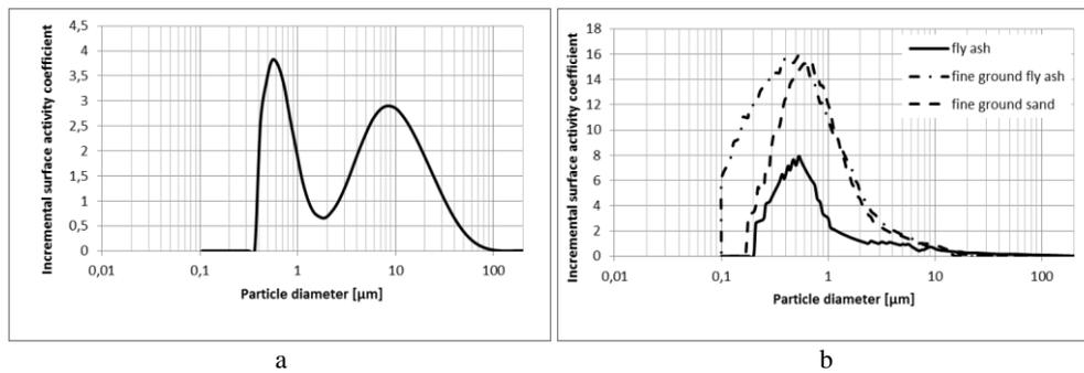
Fig. 5. Coefficient of incremental surface activity  $K_{isa}$  of cement (a) and SCMs (b)
