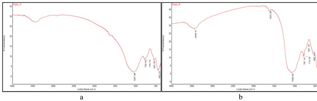
Fig. 9. Transmission spectrum of fly ash (a) and finely ground fly ash (b)
