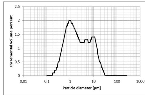
Fig. 4. The incremental volume percent of finely ground sand particles
