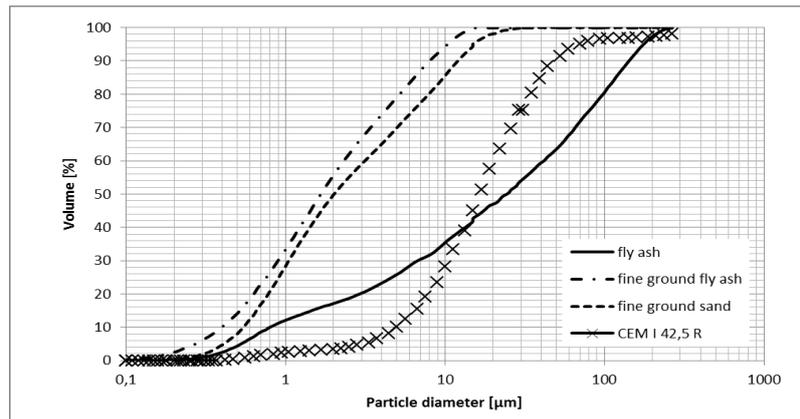
Fig. 2. Particle size distribution of cement and SCMs
