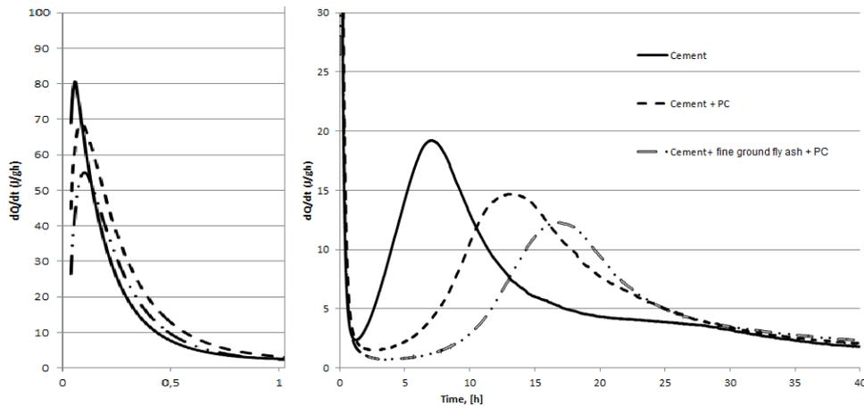
Fig. 7. Heat evolution during the hydration of Portland cement with SCMs
