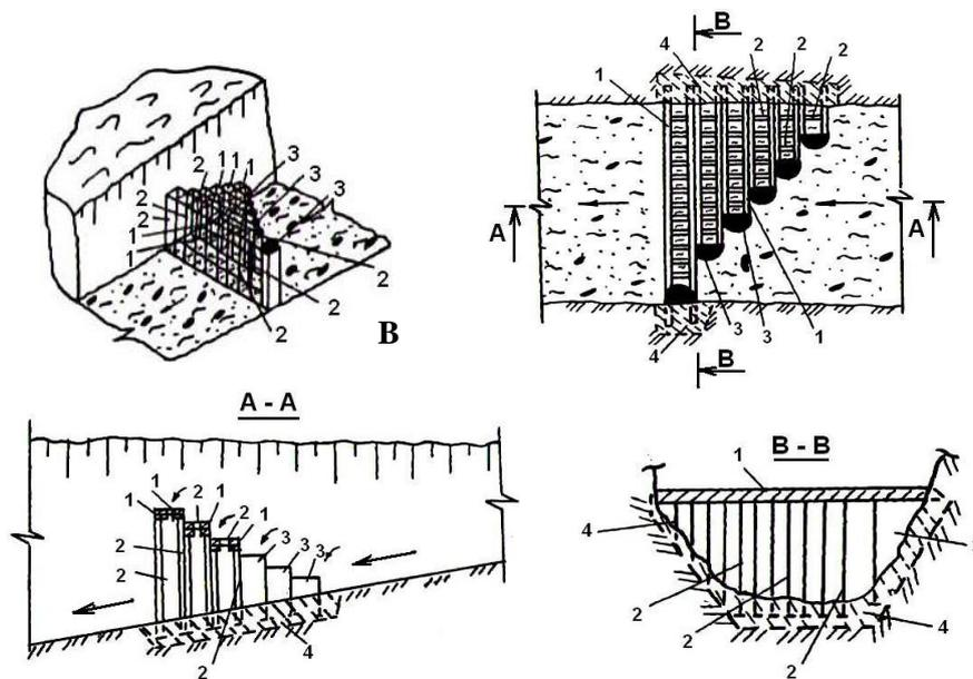
Fig. 1. Step debris control barrage
