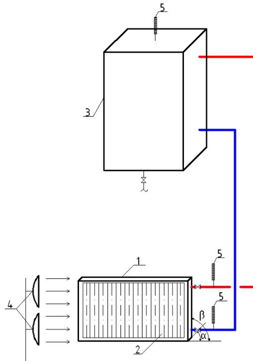
Fig. 2. Chart of the experimental unit: 1 - solar roof, 2 - accumulator box, 3 - source of radiation, 4 - mercury thermometer
