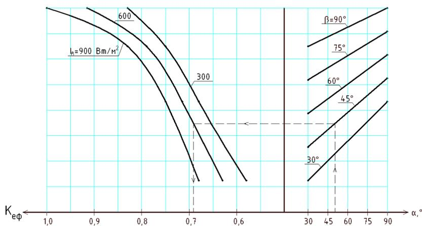
Fig. 3. Nomogram. The dependence of the efficiency of solar  $\alpha$ ,  $\beta$  and  $I_b$
