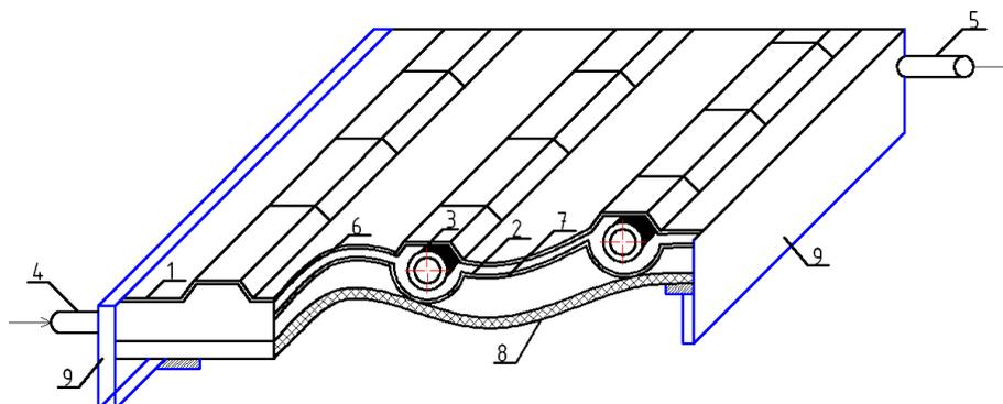
Fig. 1. Scheme of solar roof: 1 - top hose cover, 2 - bottom hose cover, 3 - tube circuits, 4 - input pipe, 5 - output pipe, 6 - selective layer material, 7 - mirror coating, 8 - insulating layer, 9 - chevron
