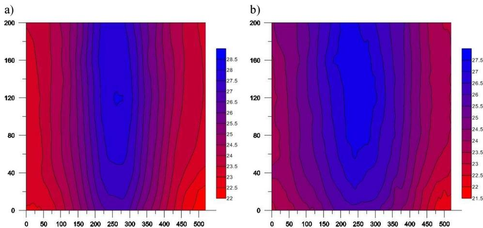
Fig. 3. The distribution of the radiation intensity radiant heater at a height of 2,8 m:
