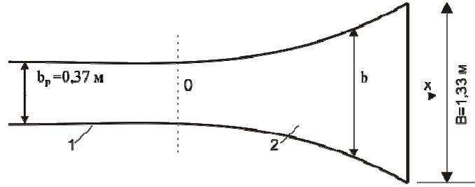
Fig. 1. The plan of the experimental model of the new facility design: 1 - prismatic channel with slope  $I = 0.03$ , 2 - non-prismatic, expanding channel with slope  $i = 0.01$
