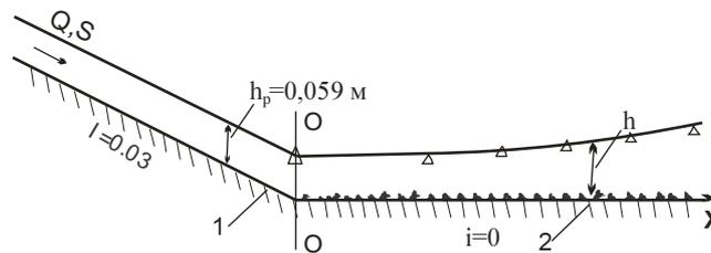
Fig. 4. Longitudinal profile of the structure - - design curve of the free surface of the flow;  $\Delta$  - experimental data; 1 - prismatic channel with slope  $I = 0.03$ , 2 - prismatic channel of reinforced roughness with slope  $i = 0.0$
