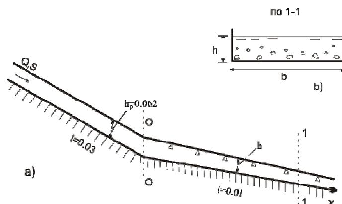
Fig. 2. The longitudinal profile (a) and the cross-section (b) of the sediment passing structure of a new design - the calculated curve of the free surface of the stream;  $\Delta$  - the results of experimental studies
