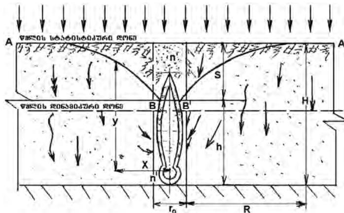
Fig. 6. Calculation plan of the combined three-tier drainage
