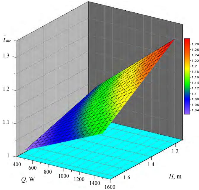
Fig. 3. Experimental dependence of the relative air temperature  $\bar{t}_{air}$  of the heater thermal capacity  $Q$  [W] and height of installing the heater  $H$  [m]
