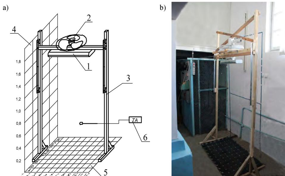
Fig. 1. Schematic of the experimental setup: a) scheme of experimental setup, b) photo of experimental setup: 1 - infrared heater NL - 12R, 2 - axial fan, 3 - tripod, 4 - vertical coordinate grid, 5 - horizontal coordinate grid, 6 - thermo-anemometer ATT-1004
