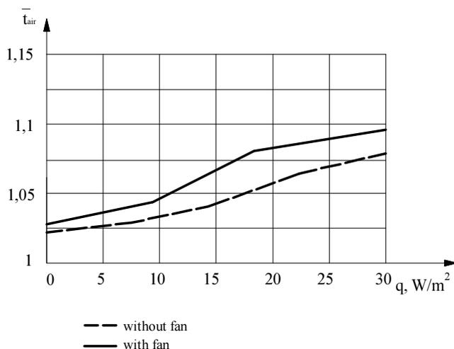
Fig. 2. Graphical dependence of the relative air temperature  $\bar{t}_{air}$  of the density of heat flow of emitter  $q$ ,  $\text{W}/\text{m}^2$  at an installation height of a heater  $H = 1.73$  m
