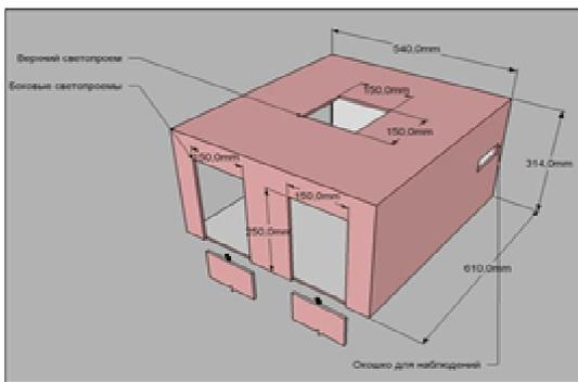
Fig. 2. The model standard room with a vertical window to evaluate the reflected light flowing into the horizontal photocell
