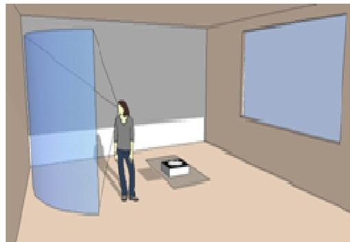
Fig. 3. The viewing angle of comfortable vision amounts near 30° up and 40°
