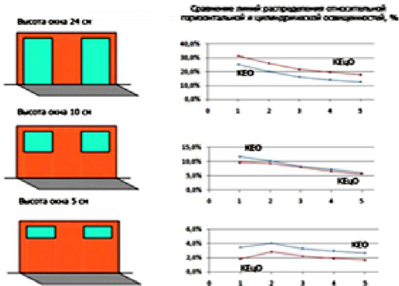
Fig. 4. The graphics of relative horizontal and cylindrical illuminations in the room with vertical windows
