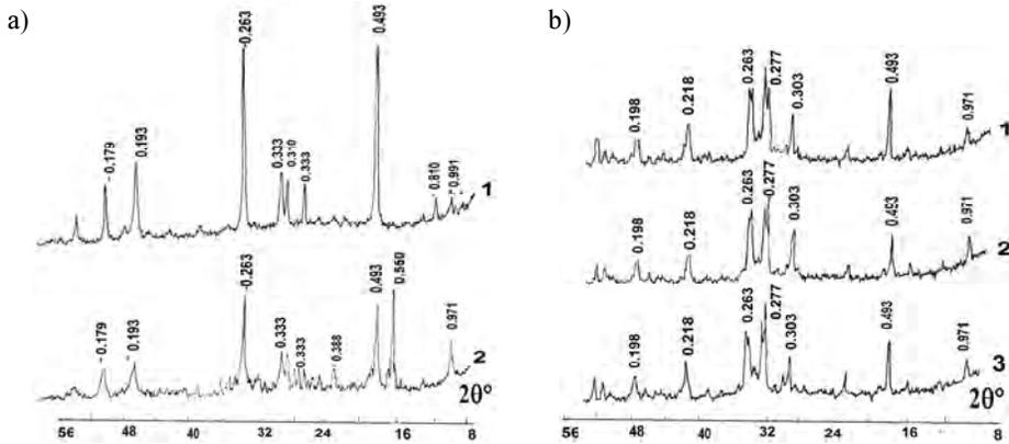
Fig. 3. XRD of the interaction products in the model systems with water after 2 days: 1 -  $\text{Ca}(\text{OH})_2$ :MK (1:1); 2 -  $\text{Ca}(\text{OH})_2$ :MK: $\text{Na}_2\text{SO}_4$  (1:1:0.5) (a) and XRD of cement pastes after 24 h of hydration: 1 - OPC; 2 - NPC; 3 - NPC\* (b)
