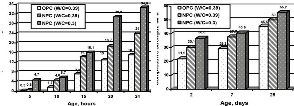
Fig. 1. Compressive strength of fine-grained concretes (C:S = 1:3) based on OPC and nanomodified Portland cement compositions
