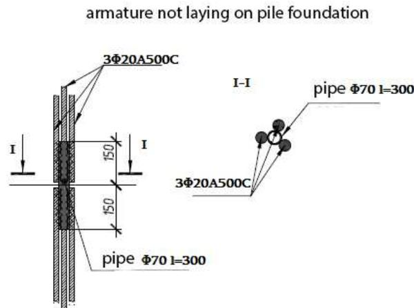
**Fig. 6.** Drill-injection pile foundation construction drilling the well is further done by dropping the reinforcement into the well and filling it with cement mortar (solution) (own study)
