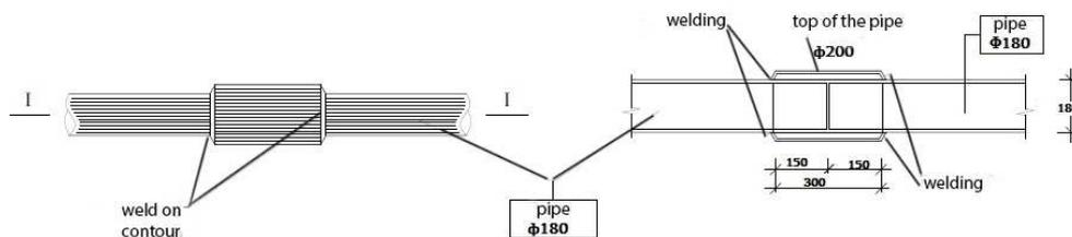
Fig. 4. Reinforcement of drill-injection pile foundations by means of injection pipe sections (own study)
