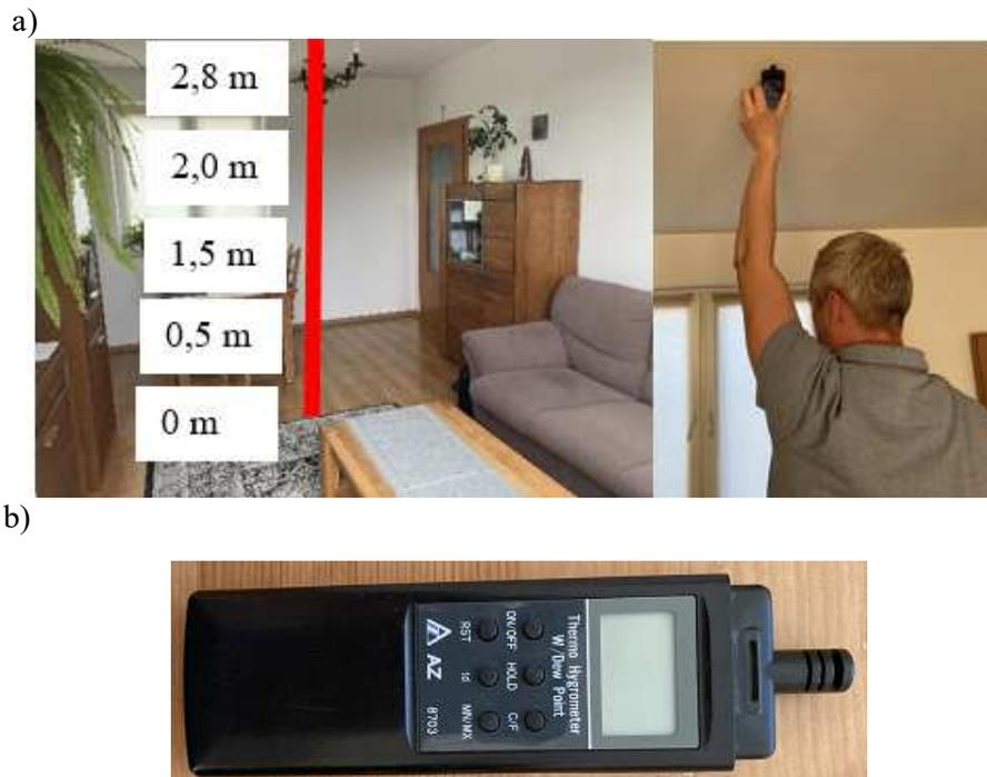
**Fig. 3.** Temperature and humidity measurement: a) measuring place, b) AZ model 8700 hygrometer (*own photo*)
