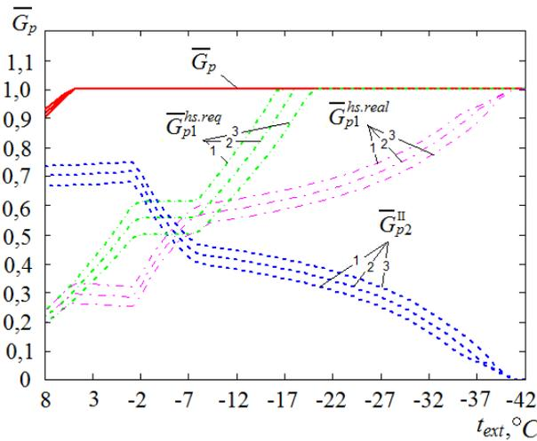
**Fig. 2.** Relative flow rates of network water in heat points; 1 –  $\psi = 0.5$ ; 2 –  $\psi = 0.63$ ; 3 –  $\psi = 0.79$  (Rafalskaya et al., 2017)
