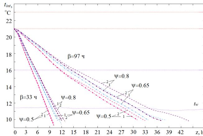
**Fig. 9.** Indoor air temperature, January 14-17, 2018; 1 – at the working second stage of the hot water heater; 2 – at turning off second stage of the hot water heater (*own research*)
