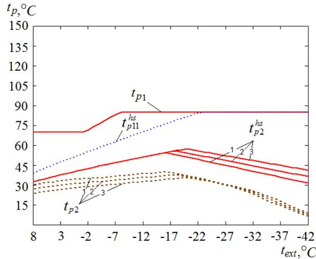
**Fig. 1.** Water temperature in the heat supply system during emergency operation of the CHP; 1 –  $\psi = 0.5$ ; 2 –  $\psi = 0.63$ ; 3 –  $\psi = 0.79$  (Rafalskaya et al., 2017)
