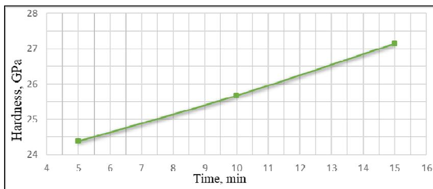
**Fig. 2.** Dependence of hardness of a covering on spraying time (*own study*)
