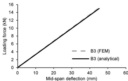
Fig. 4. Deflection vs. load diagram for a beam reinforced with two tapes glued to the last lamella (*own study*)
