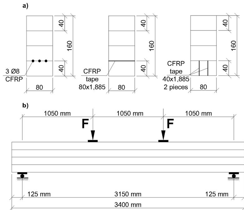
**Fig. 1.** Assumptions adopted for numerical simulations: a) analyzed cross-sections, b) static diagram adopted for numerical models (based on Jończyk, 2019)
