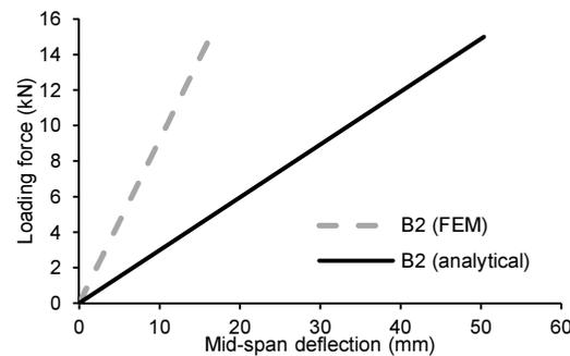
Fig. 3. Deflection vs. load diagram for a beam reinforced with one tape (*own study*)
