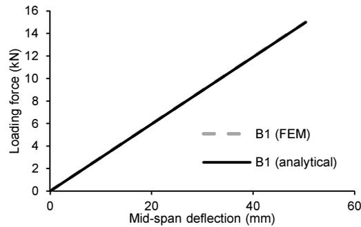
Fig. 2. Deflection vs. load diagram for a three-bar reinforced beam (*own study*)
