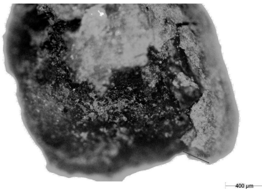
**Fig. 2.** Photograph of the grain of the catalytic mass together with a cracked shell from accumulated sludge (*own research*)
