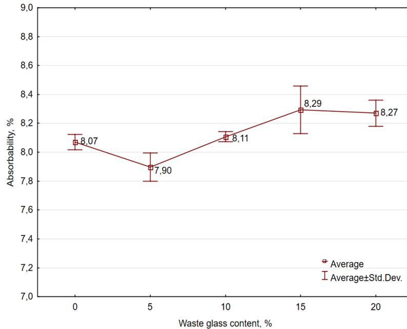
**Fig. 5.** Function graph describing the dependence of absorbability on the percentage share of glass waste in mortar (*own research*)
