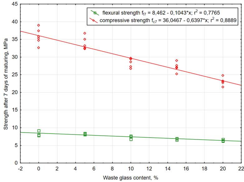
**Fig. 3.** Function graphs describing the dependence of flexural and compressive strength after 7 days of maturation on the percentage of glass waste in mortar (*own research*)
