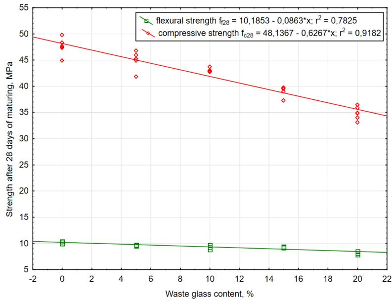
**Fig. 4.** Function graphs describing the dependence of flexural and compressive strength after 28 days of maturation on the percentage of glass waste in mortar (*own research*)
