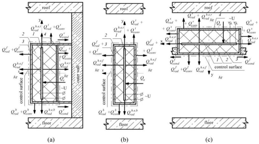
**Fig. 1.** The scheme of heat flows in radiant heating panels of different alignment: 1 - metallic heating element, 2 - thermal and electrical insulator, 3 - framework, 4 - shielding plate
