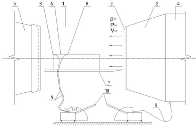
Fig. 1. Diagram of experimental installation of residential complex model in aerodynamic tube: 1 - working part of aerodynamic tube, 2 - nozzle, 3 - alignment grid, 4 - fire chamber, 5 - diffuser, 6 - residential complex model, 7 - model substrate surface, 8 - selected static pressure points, 9 - flexible tubes, 10 - micromanometer
