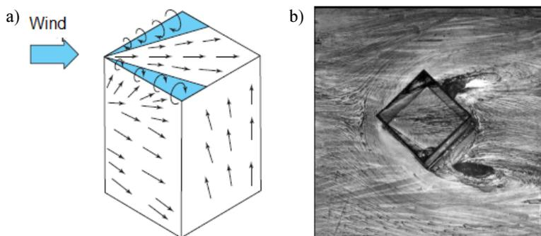
Fig. 3. Distribution of air flows that arise at a wind load directed at angle of  $45^\circ$  to building facade: a) scheme of air flows [8], b) results of soot-oil visualization [9]
