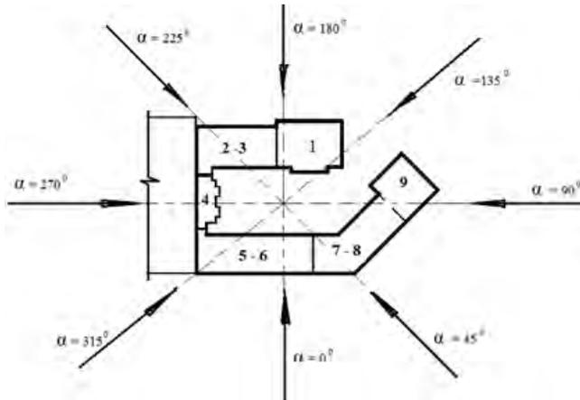
Fig. 2. Angles of attack on residential complex model
