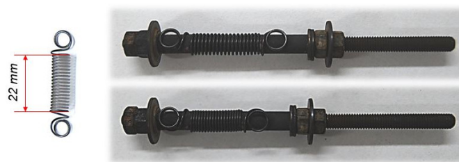
Fig. 2. Fixture with the SMA spring subjected to annealing at different temperatures ( own research )
